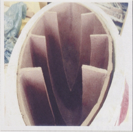
Fig.37 Attaching the interior structure called 'webbing', that keeps the walls from buckling. The webbing should be curved, since a curve can respond to stresses by bending.
