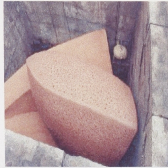
Fig.50 Placing the bisqued forms inside the black firing kiln, ready for the reduction process.
