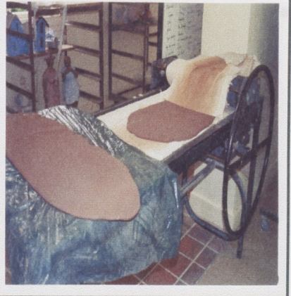
Fig.34 Making clay slab from a slab roller machine, the most convenient and a tremendous work saver.
