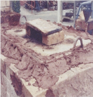
Fig.51 Sealing the lid of the kiln with clay slurry.
