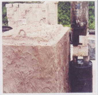
Fig.54 Dripping of the sump oil from a tank placed beside The kiln. The entire kiln is sealed further with slurry to ensure total reductio.
