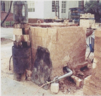
Fig.53 The kiln is fired to 800°C, upon reaching this temperature, the gas burner is turned off.
