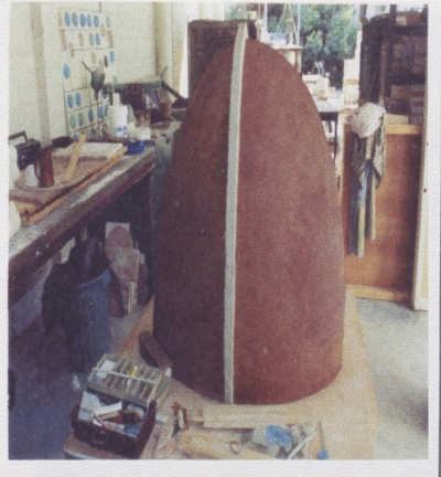
Fig.26 Attaching a shim made from clay slab for the parting line; the mold must separate along the line.
