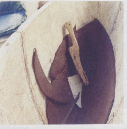
Fig.35 Pressing the layer of clay slab over the entire inner surface.
