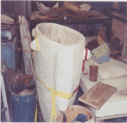
Fig.33 Strapping the two-piece mold together after drying and bracing it firmly.
